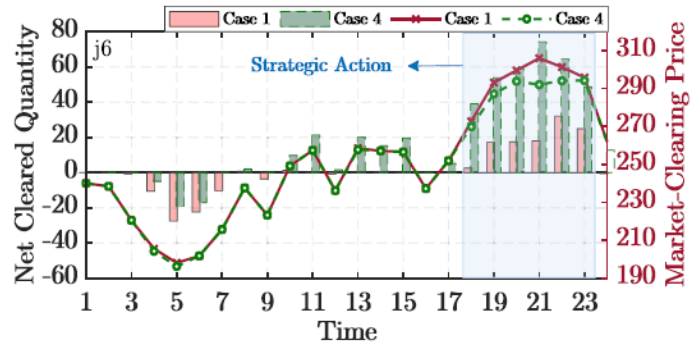
Figure - Hourly hybrid storage commitment (bars, MW) and market-clearing price (lines, €/MWh) on day 6
