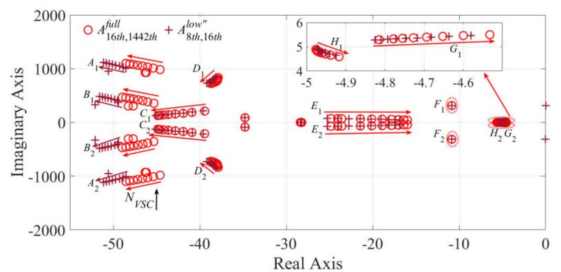
Eigenvalues loci of the full-order (symbol O) and reduced-order (symbol +) SSMs when paralleled branches increases from 4 to 32 with step size 4.
