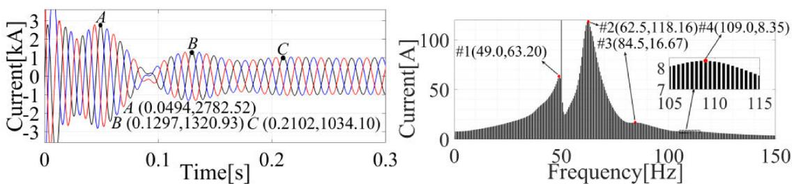
Time-domain simulation results of three-phase output currents of VSC #1. (a) Waveform and (b) FFT. (#1, #2, #3, #4 correspond to  $G_{1,2}$ ,  $E_{1,2}$ ,  $C_{1,2}$ , and  $B_{1,2}$ , respectively.)
