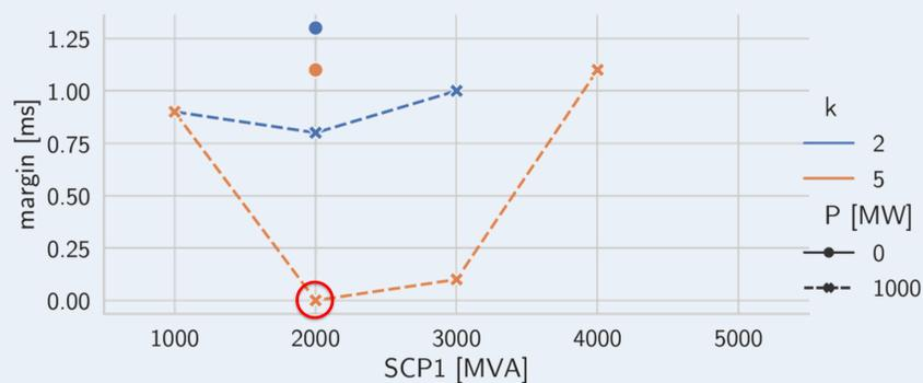
The smallest time margin between forward and (incorrect) reverse detection functions occurs for: a weak local bus and fast fault current injection with a large injection factor.
