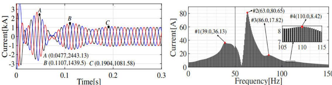
Time-domain simulation results of three-phase output currents of VSC #1. (a) Waveform and (b) FFT as the PLL parameters of the four VSCs are increased.
