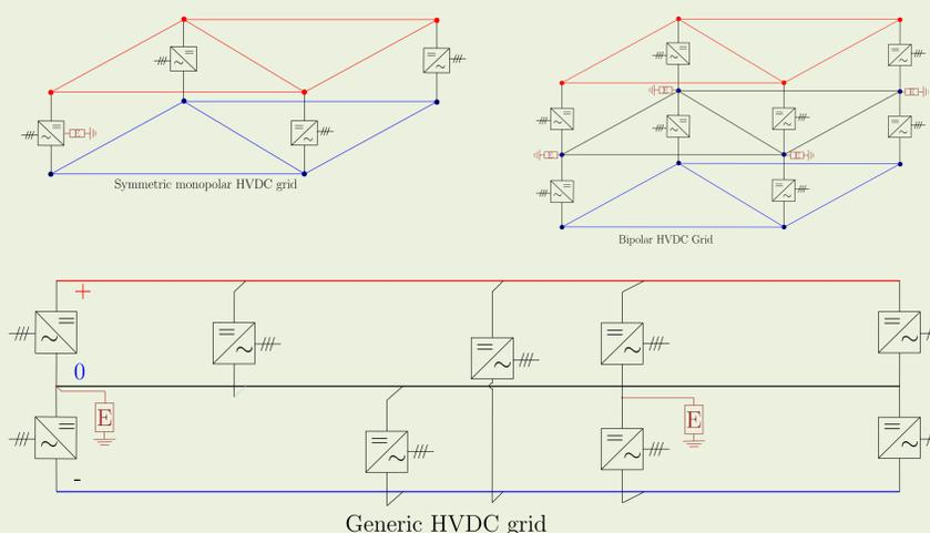
Operation of the system with mixed configurations would create unbalance in the DC grid. The mixed configurations can occur either by grid design or in case of contingencies.
