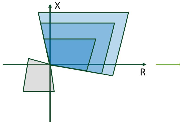
$$\underline{Z} = x\underline{Z}_l + R_f + \frac{I_2}{I_1} R_f$$
