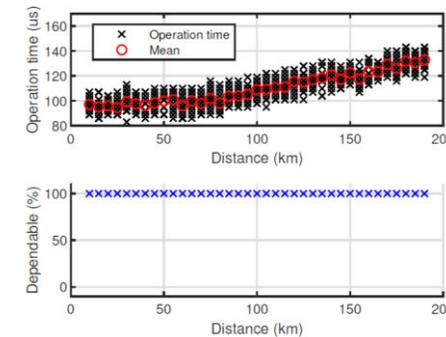
(b) Dependability for faults in protection zone (Cable L1)
