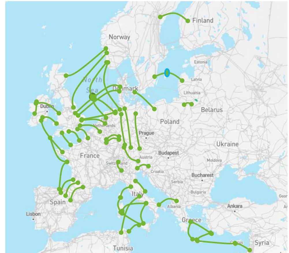
Subset of HVDC connections in TYNDP 2020 of ENTSO-E
