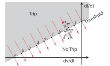
(a) Algorithm characteristic and perpendicular test ramps
